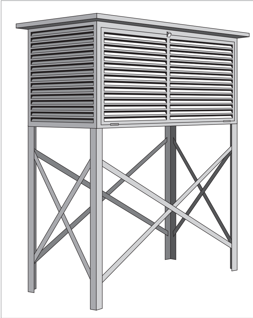
Stevenson screen. A Stevenson screen is a container of standard construction that is used to house the thermometers used at a weather station. The screen is painted white, has double-louvered sides, and is sited in the open well clear of the ground.
