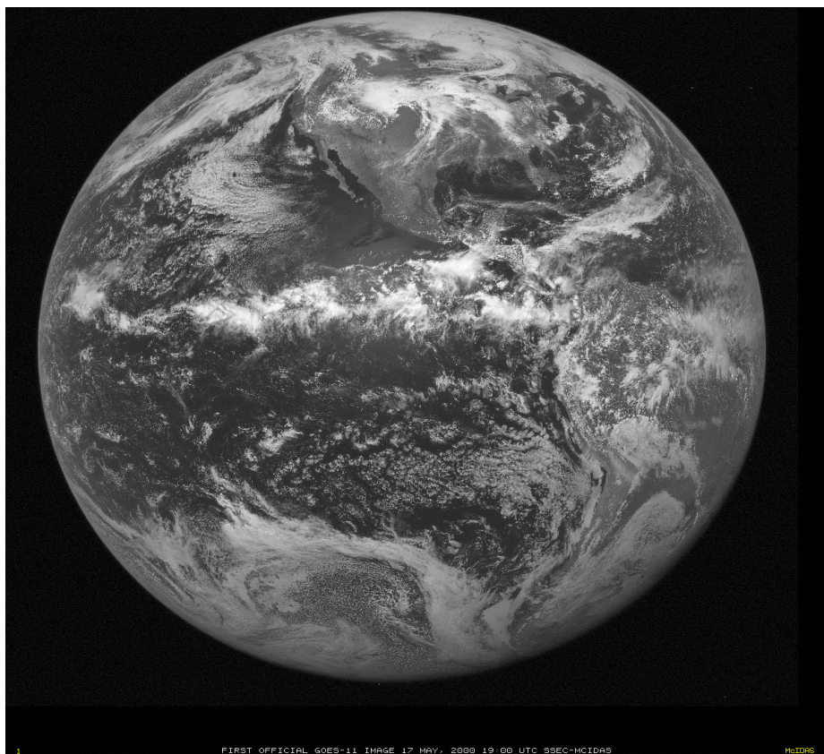
Figure 1.4. Image of visible reflectance sensed by the GOES-11, in which the light areas correspond to clouds or snow/ice regions.
